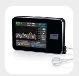
The Tandem t:slim can hold up to 300 units of insulin, which it administers according to the readings taken by a connected Continuous Glucose Monitor (CGM). It works by delivering insulin directly into the body via an infusion set or tubing system. There are several infusion sets to choose from so you can find what works for you. The t:slim has a rechargeable battery and a touch colour screen, plus sleep and exercise modes.
